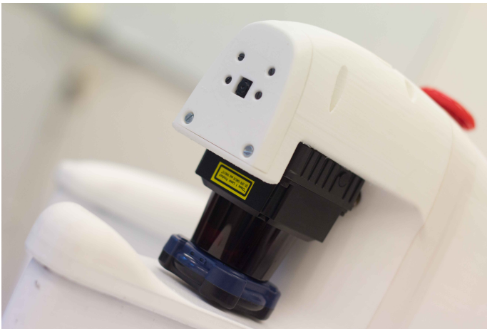
Fig. 3: Lidar and Camera placement
